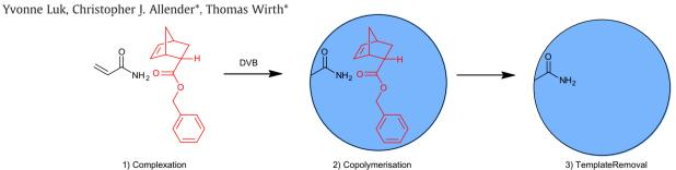
A series of highly specific molecular imprinted polymer (MIP) imprinted with a small, low functionality and bicyclic *endo*-product of a Diels-Alder reaction was prepared. The selectivity of the MIPs was evaluated on the basis *endo/exo* discrimination.
